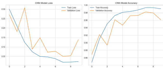
Figure 6. Training and Validation History for the EfficientNetV2-S Model, showing Loss and Accuracy over 10 epochs.
